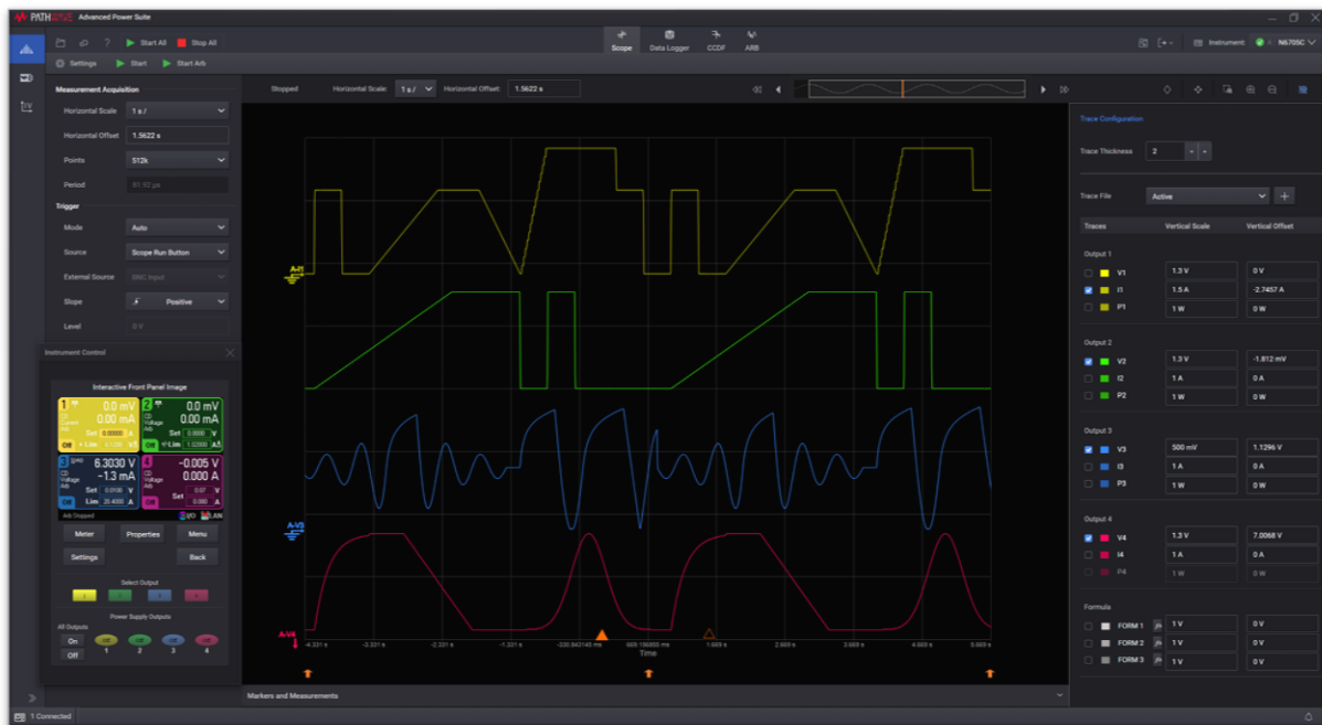
Figure 5. PW9252A interface with 4 channels connected
