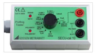
All limit values for the required tests per DIN VDE must be tested, such as protective conductor resistance, insulation resistance, equivalent leakage current, differential current and/or contact or housing leakage current.
