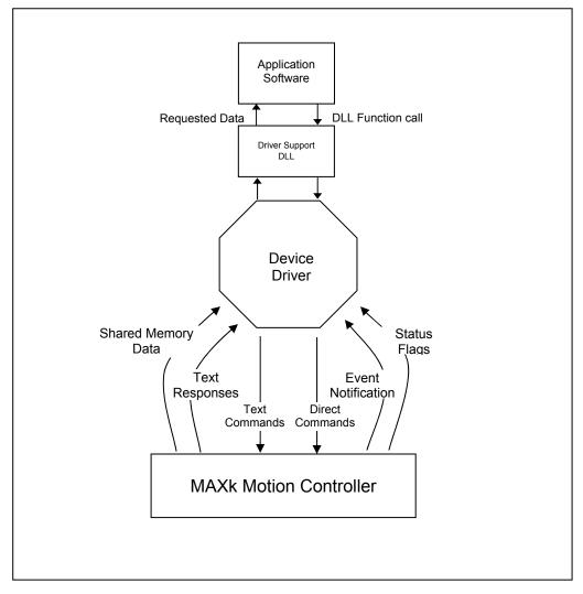
Figure 3-1 FUNCTIONAL COMMUNICATIONS FLOW
