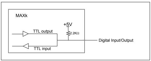
Figure 4-4 GENERAL PURPOSE I/O WIRING DIAGRAM
