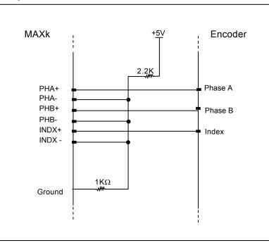
Figure 4-5 ENCODER HOMING STATE DETECTION
