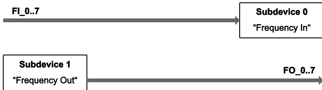
Diagram 7: Frequency input/output in single operation mode
