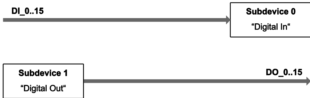
Diagram 9: Digital input/output in single operation mode
