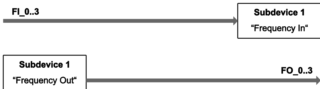
Diagram 17: Frequency input/output in single operation mode
