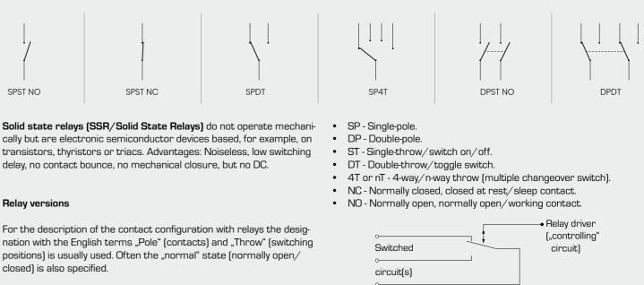
cally but are electronic semiconductor devices based, for example, on transistors, thyristors or triacs. Advantages: Noiseless, low switching delay, no contact bounce, no mechanical closure, but no DC.
