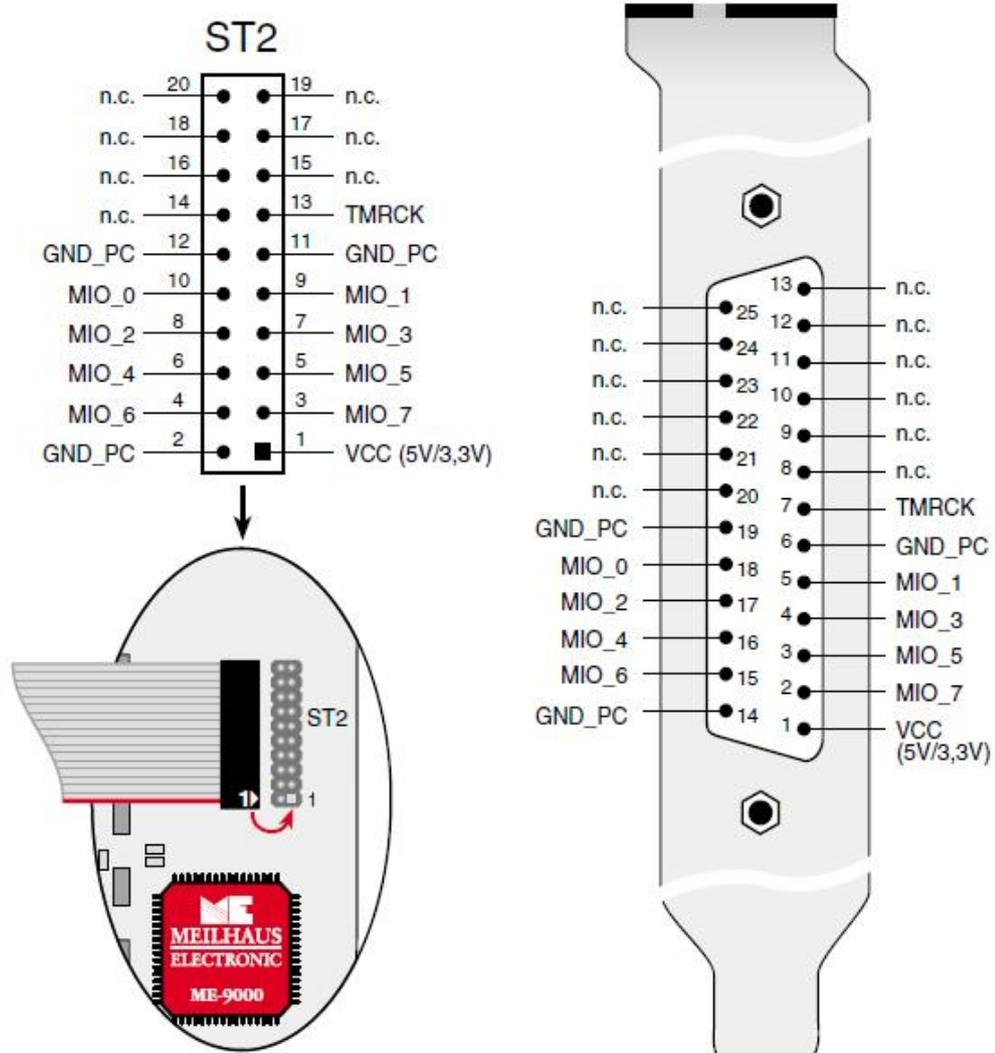
Picture 62: Pinout of ST2 on ME-9000 (i)
