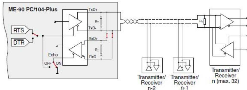
Picture 50: Operation mode "RS-485 half-duplex" ME-90 PC/104-Plus
