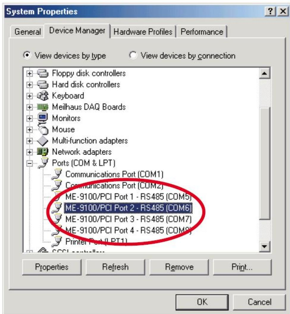
Picture 1: Entry of ports in the device manager
