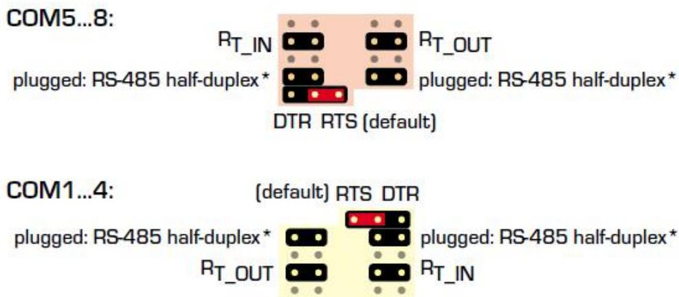
Picture 31: Jumper for port configuration ME-90 PC/104-Plus
