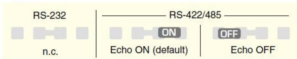
Picture 32: Soldering bridges ME-90 PC/104-Plus
