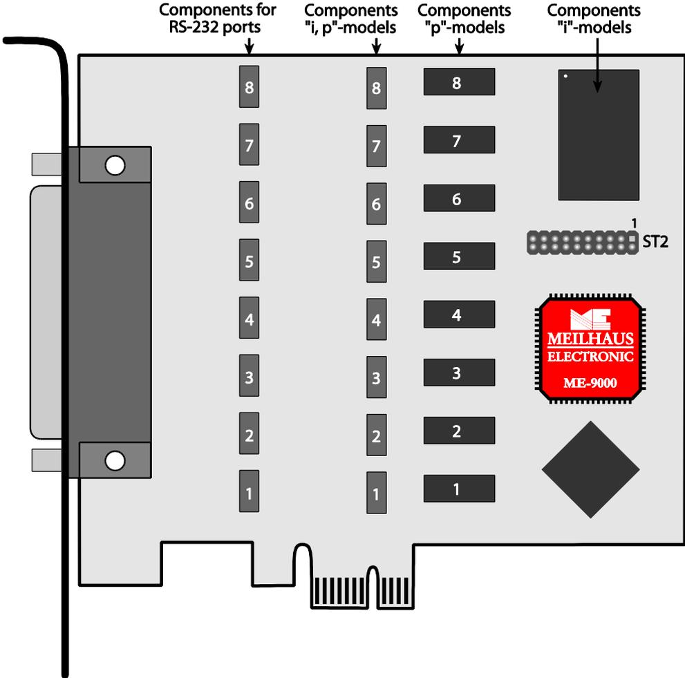
Picture 18: ME-9000 Compact PCI Rev. 2.2 (top view)
