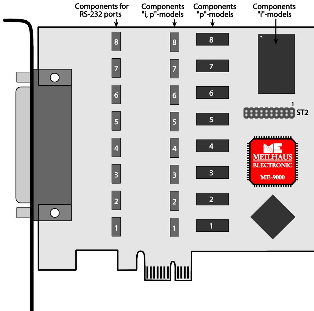
Picture 16: ME-9000 PCI Rev 2.2 (top view)
