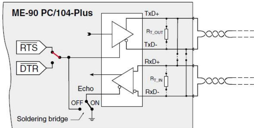
Picture 30: Configuration RS-422/485 ports ME-90 PC/104-Plus
