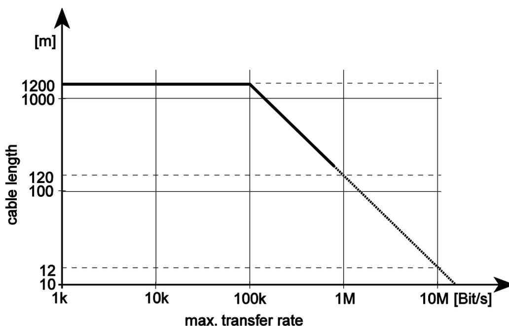
Picture 44: Dependency of cable length to max. transfer rate with terminated lines
