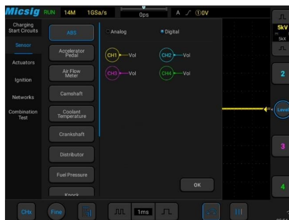
▲ Directly measure the waveform of various Sensors, by comparing with standard waveform, helps user easily find out possible problem.
