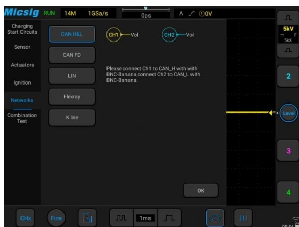
▲ SATO is capable of acquiring and decoding CAN High /CAN Low, CAN FD, LIN, FlexRay, and K line signals, delivers professional Network communication tests on vehicles.
