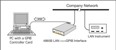
Figure 3 4865B Instrument Network Connection
