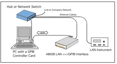
Figure 2 4865B Instrument Hub Connection
