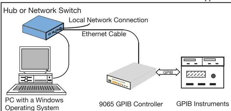
Figure 1 9065 shown connected to Company Network
