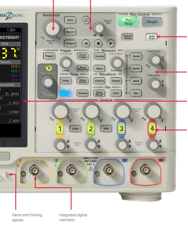
Autoscale lets you quickly display any analog or digital active signals, automatically setting the vertical, horizontal and trigger controls for the best display, while optimizing memory
