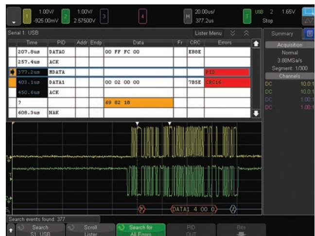
Figure 21. USB 2.0 trigger, decode and "lister" display.
