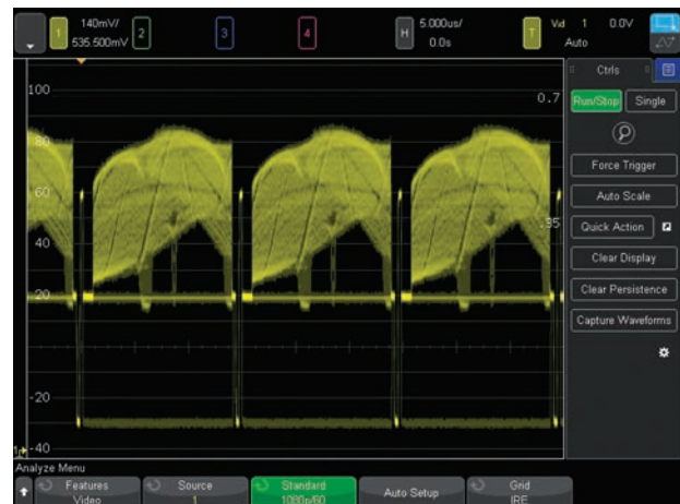
Figure 27. Triggering on 1080p HDTV signal analysis.
