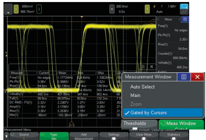
Figure 33. Up to 10 automated measurements displayed simultaneously. Measurements can be gated by cursors.
