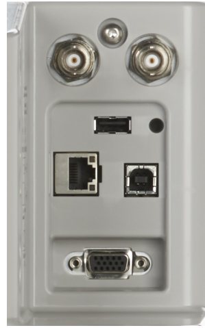
Figure 52. Connectivity section on the back panel.
