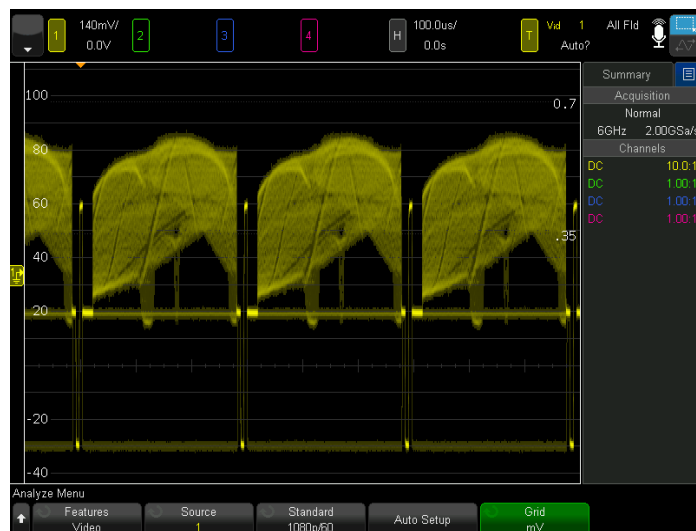
Figure 45. Triggering on a 1080p/60 signal.
