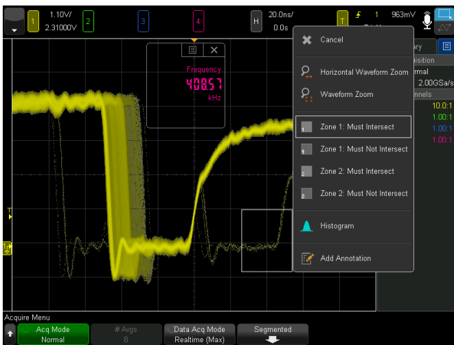
Figure 11. Draw a zone (box) around the anomaly.
