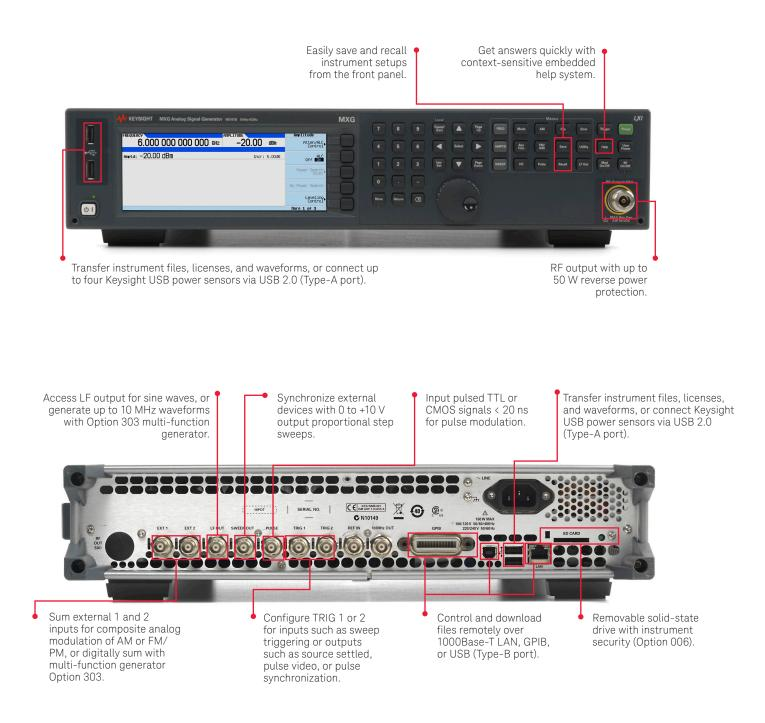
Note: The MXG and EXG X-Series analog signal generators have the same connector layout.
