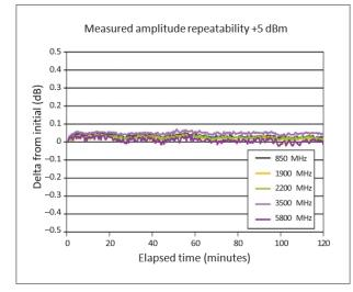
Repeatability measures the ability of the instrument to return a given power setting after a random excursion to any other frequency and power setting. It should not be confused with absolute level accuracy.
