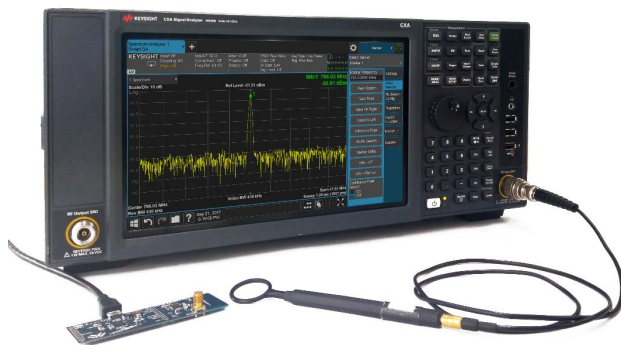
Figure 8. Detecting EMI emissions with a near-field probe (N9311X-100)
