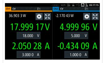
The linear design of the output stages reduces residual ripple and noise to a minimum and makes it perfect to support the development of power amplifiers and MMICs.
