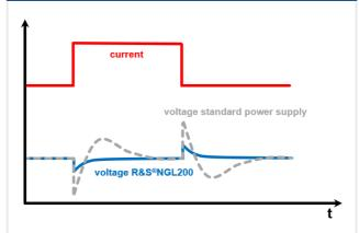
During challenging load conditions, most power supplies react with slow recovery times and overshoots. Specially developed circuits in the R&S\*NGL200 series achieve a load recovery time of  $<30~\mu s$  with minimal overshoot, making them perfect for supplying sensitive components
