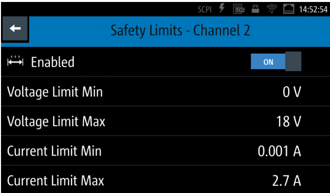
The user can set safety limits to limit the adjustment range of the power supply and prevent a DUT from being damaged due to accidentally using the wrong setting.
