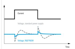
Under challenging load conditions, most power supplies respond with slow recovery times and overshoots. Specially developed circuits in the R&S\*NGM200 power supplies achieve a load recovery time of  $<30~\mu s$  with minimal overshoot, making them perfect for supplying sensitive components.
