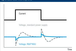
Under challenging load conditions, most power supplies respond with slow recovery times and overshoot. Specially developed circuits in the R&S°NGU source measure units achieve a load recovery time of  $<30~\mu s$  with minimal overshoot, making them perfect for supplying sensitive components with power.
