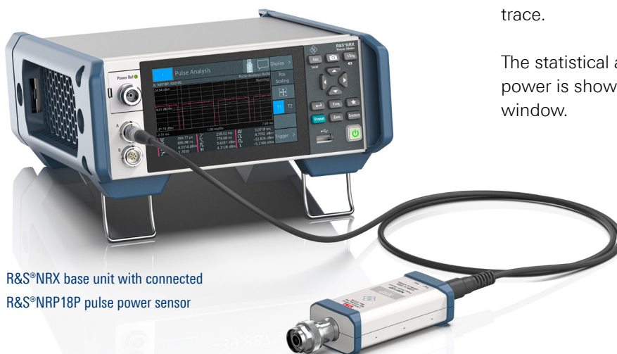
Automatic pulse analysis with the R&S®NRX and R&S®NRP18P
