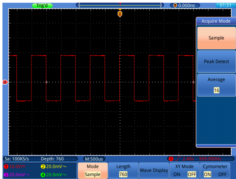
Figure 0-3 Normal ACQU Mode display, in which no burr can be detected.
