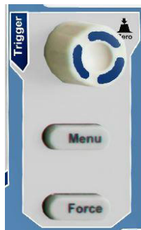
Figure 3-12 Trigger Control Zone
