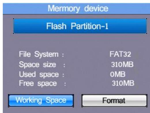
Press the ◀ and ▶ button to select the Working Space or Format. Then press the □ button to enter, press the ESC button to esc and save.
