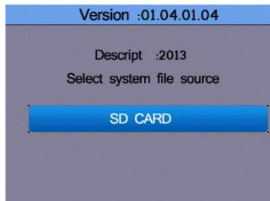
If a firmware update is available, this can be stored on an SD card and are available as a source for an update is available. Firmware updates should only be performed by qualified personnel as an incorrect application may damage the unit.
