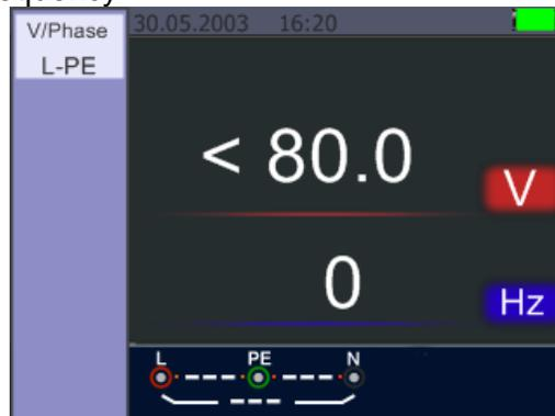
Standby screen for the Voltage and Frequency
