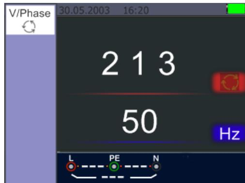
**Phase Sequence – When connected in counter-clockwise manner**
