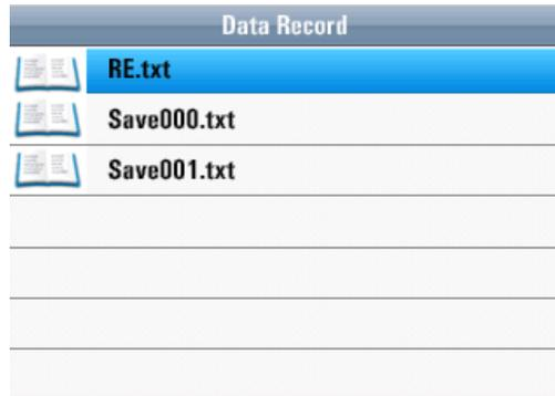
In the Data Record menu, you see a list of previously stored measurement values to a text file for single values or data logger files. Press the ▲ or ▼ keys to scroll through the menu and confirm your selection by pressing the □ button (Enter). The following screen appears after selecting a stored file:
