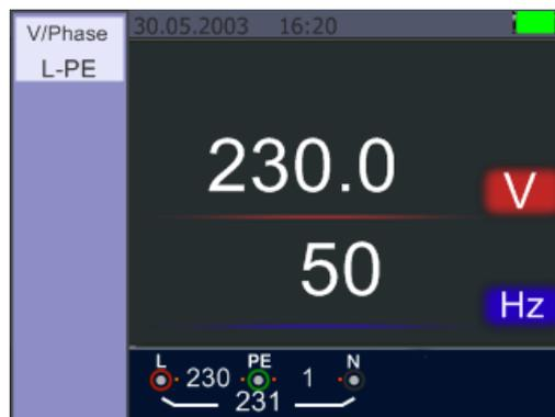
Screen while measuring Voltage and Frequency
