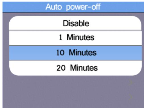
Default 10 Minutes, Press the ▲ and ▼ button to select the Auto power-off time, press ESC button to esc and save the select the time.
