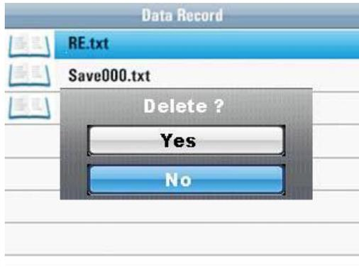
Use the ▲ or ▼ buttons to select YES (YES) or NO (NO) and confirm the deletion by pressing the □ button (Enter)
