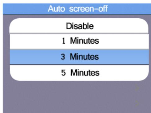
Default 3 Minutes, Press the ▲ and ▼ button to select the Auto screen-off time, press ESC button to esc and save the select the time.
