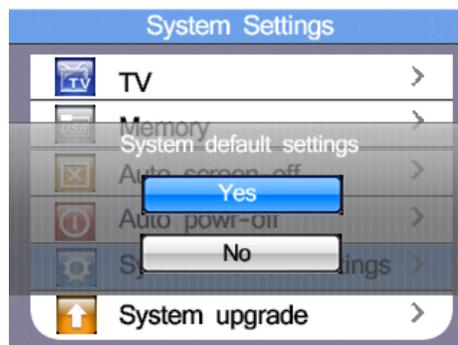
Press the □ button to enter. Then press the ▲ and ▼ button to select whether YES or NO to Reset.
