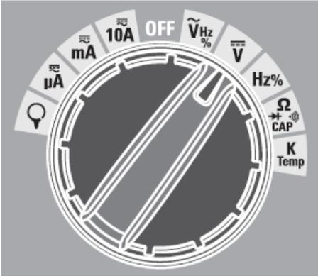
Select a primary measurement function by positioning the rotary switch to one of the icons around its perimeter. For each function, the Meter presents a standard display for that function (range, measurement units, and modifiers). Button choices made in one function do not carry over into another function.
