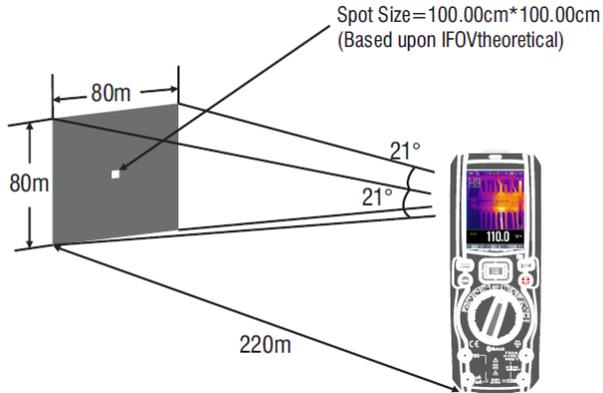
$D:S_{\text{measure}}$  ( $= 1/ \text{IFOV}_{\text{measure}}$ ) is the spot size needed to provide an accurate temperature measure. Typically,  $D:S_{\text{measure}}$  is 2 to 3 times smaller than  $D:S_{\text{theoretical}}$ , which means the temperature measurement area of the target need to be 2 to 3 times larger than that determined by the calculated theoretical  $D:S$ .
