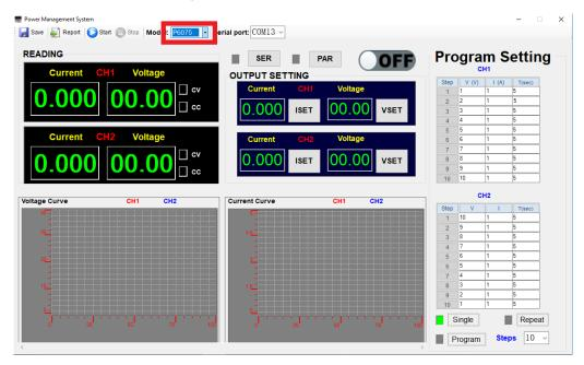
Enter the value of current and voltage into the "OUTPUT SETTING" frame (see.P2) and then click the ISET/VSET to send the value to the DC power supply. For activating the output click on the button. The appearance of the button will change to switched on.
