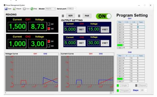
To stop the program run, click on the Stop button. The output stops at the last program step. The output keeps power on.
