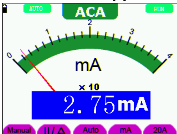
Figure 25: AC Current Measurement for 400 mA
