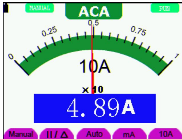
Figure 26: AC Current Measurement for 10A
