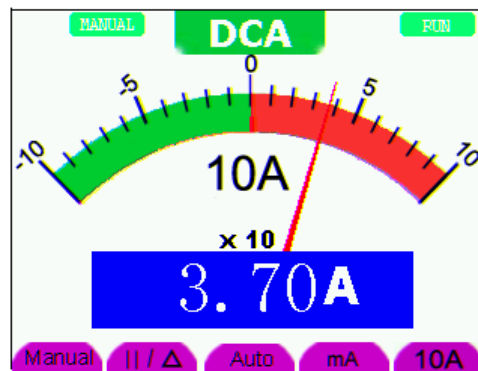
Figure 28: DC Current Measurement for <10A
