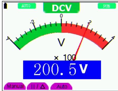
Figure 25: DC Voltage Measurement
