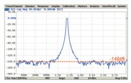
Typical dynamic range of 125 dB, typ. is achieved through the entire frequency range (10 Hz IF BW). Seen here is the maximum dynamic range achieved when using 10 IF BW and an output power level of 10 dBm.
