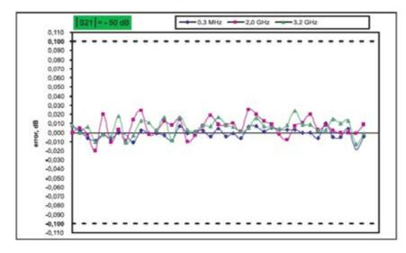
Low trace noise allows for particularly high-precision measurements. This graph shows the variation of the absolute value of the measurement error of  $S_{21}$  and  $S_{12}$  with a value of  $|S_{21}|$  and  $|S_{12}|$  -50 dB, using 42 different instruments. With the model's specifed accuracy of  $\pm$  0.1 dB, the trace clearly shows that the variations within the instrument pool is well below that figure. This confirms the precision of the instrument.
