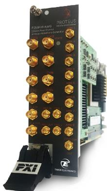
Integrated digital up-converter to RF frequencies for coherent multi-channel RF applications across multiple modules
