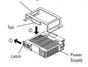
① Pull out the latch to UNLOCK position.
