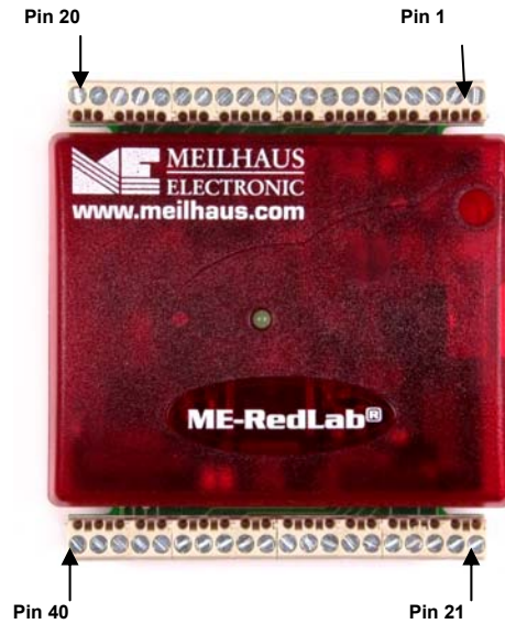
Figure 4. RedLab 1024LS screw terminal pin numbers
