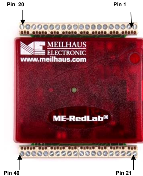
Figure 4. RedLab 1024HLS screw terminal pin numbers
