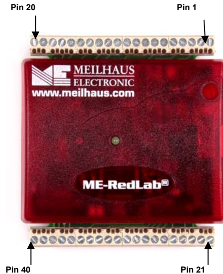
Figure 4. RedLab 1208LS Screw terminal pin numbers
