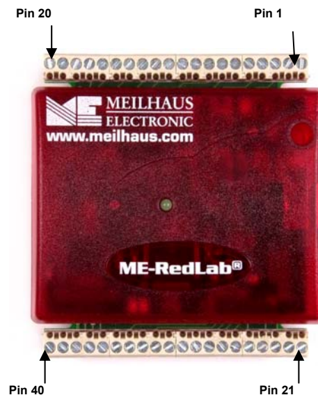
Figure 4. RedLab 1208FS Screw terminal pin numbers
