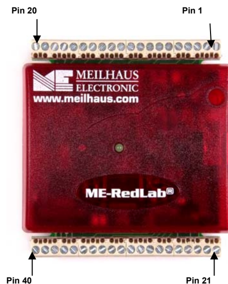
Figure 4. RedLab 1408FS Screw terminal pin numbers
