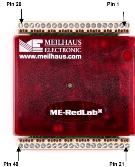
Figure 4. RedLab 1608FS screw terminal pin numbers
