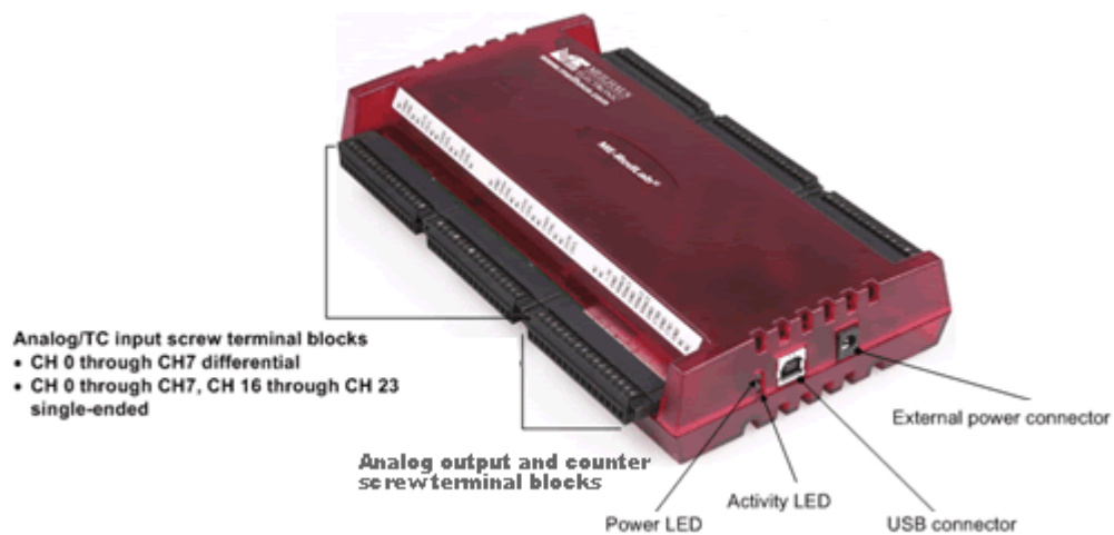
Figure 6. RedLab 2416-4AO components – front view
