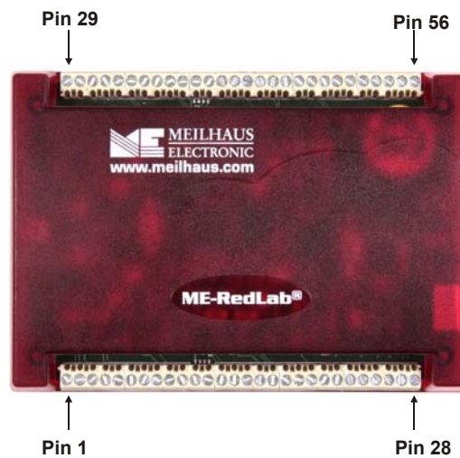
Figure 4. RedLab 3103 screw terminal pin numbering
