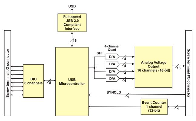
Figure 2. RedLab 3105 block diagram
