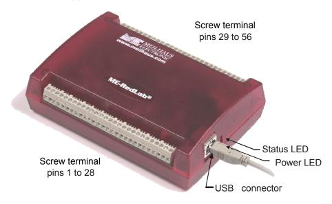
Figure 3. RedLab 3105 external components
