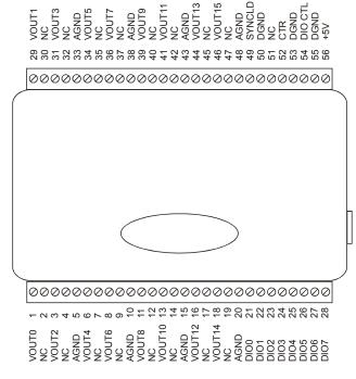
Figure 5. RedLab 3105 signal pin out
