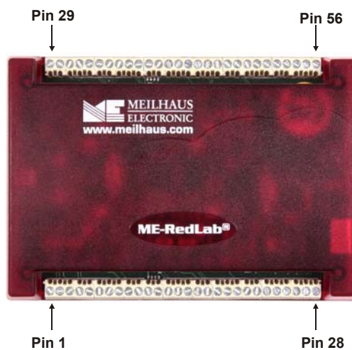
Figure 4. RedLab 3114 screw terminal pin numbering
