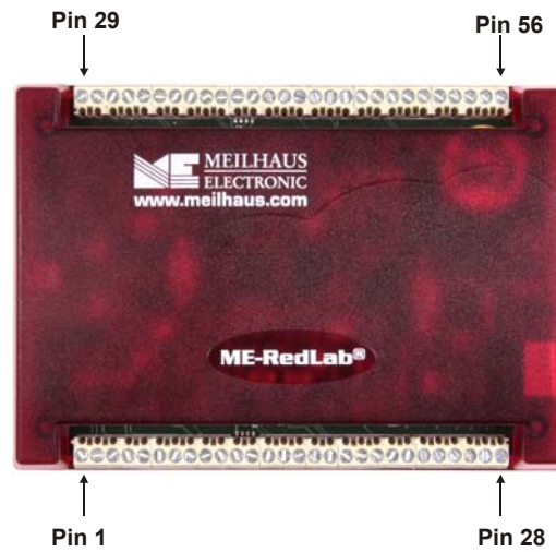
Figure 4. RedLab 3102 screw terminal pin numbering
