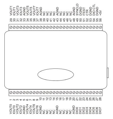
Figure 5. RedLab 3104 signal pin out
