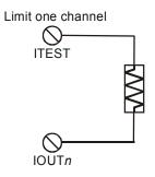
Figure 7. Current output test circuit
