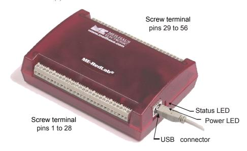
Figure 3. RedLab 3104 external components
