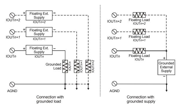
Figure 6. Typical analog current output circuit
