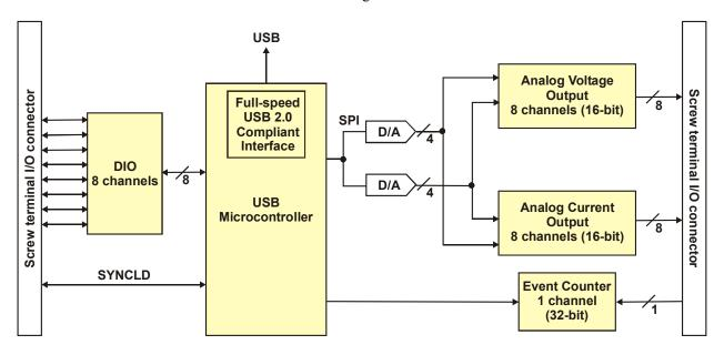
Figure 2. RedLab 3104 block diagram
