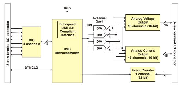
Figure 2. RedLab 3106 block diagram
