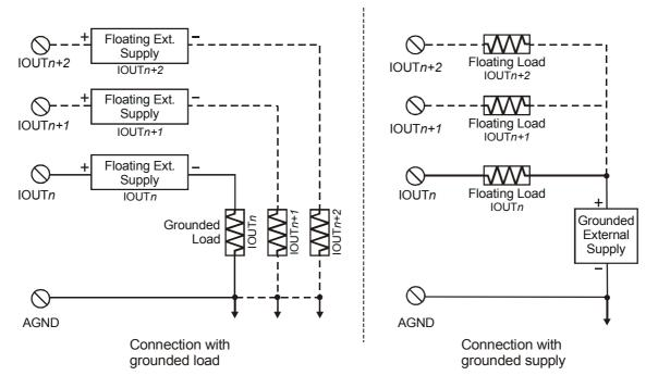
Figure 6. Typical analog current output circuit
