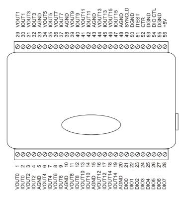
Figure 5. RedLab 3106 signal pin out
