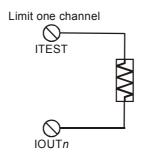
Figure 7. Current output test circuit
