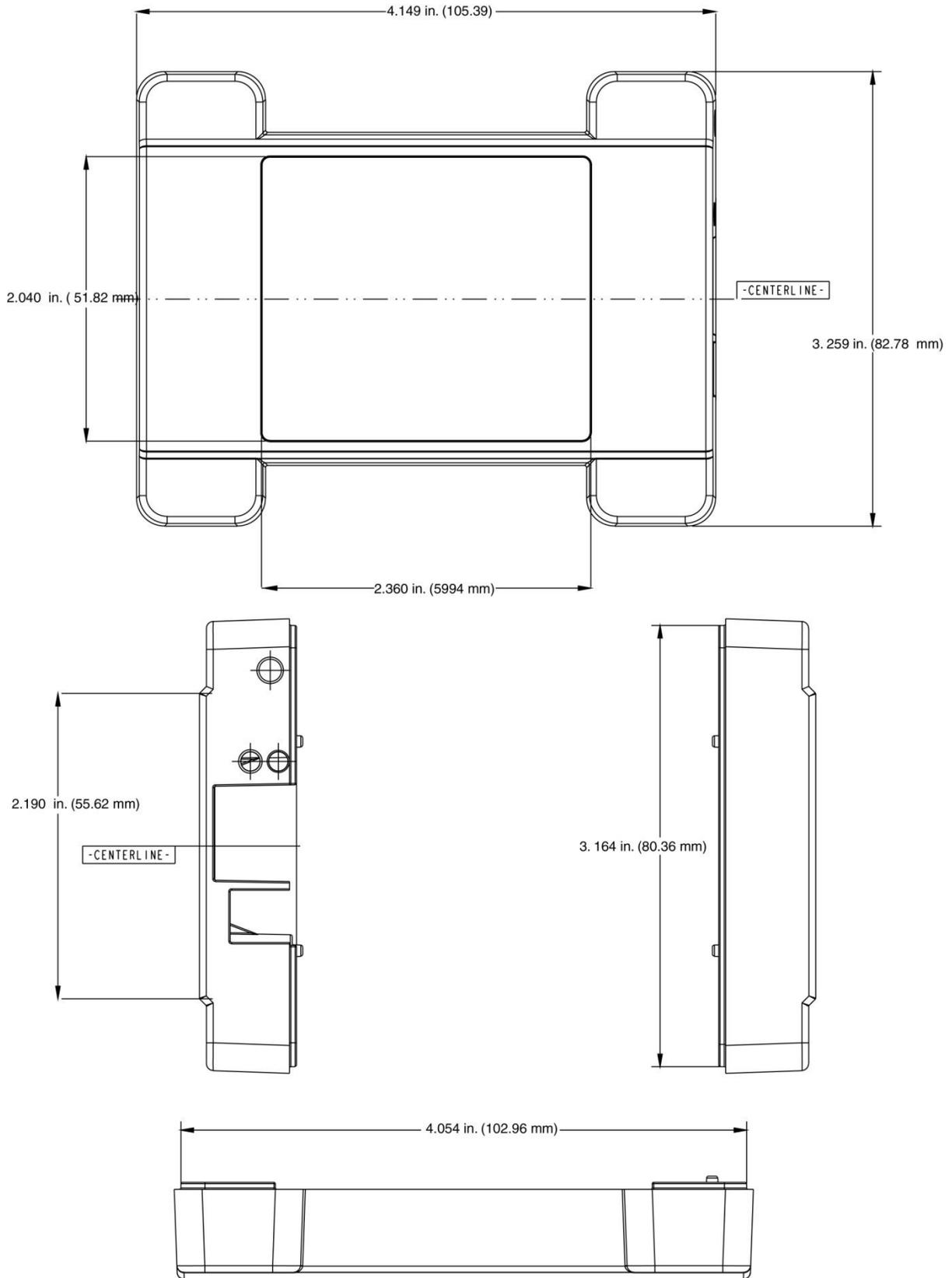
Figure 10. RedLab E-1608 top enclosure dimensions
