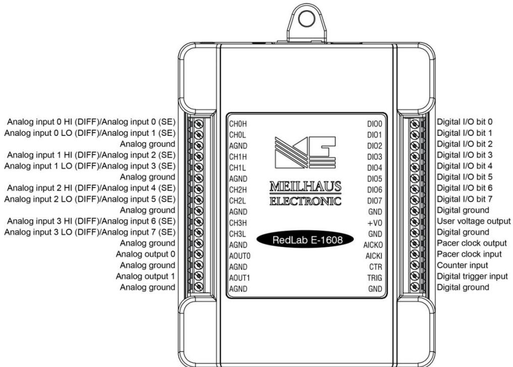
Figure 3. RedLab E-1608 pinout
