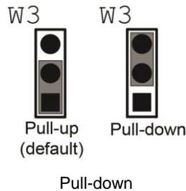
Figure 7. W3 jumper configurations
