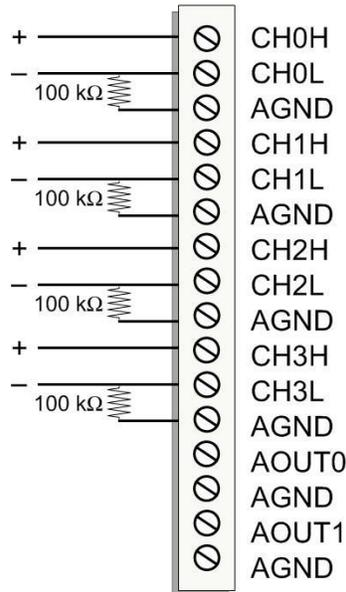
Figure 4. DIFF connections with ground path resistor
