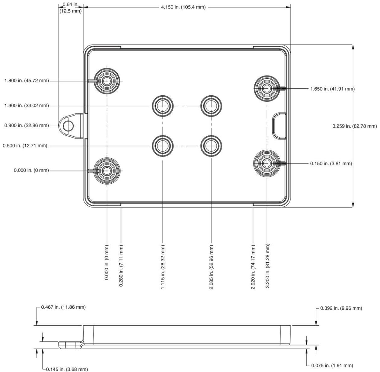
Figure 9. RedLab E-1608 bottom enclosure dimensions
