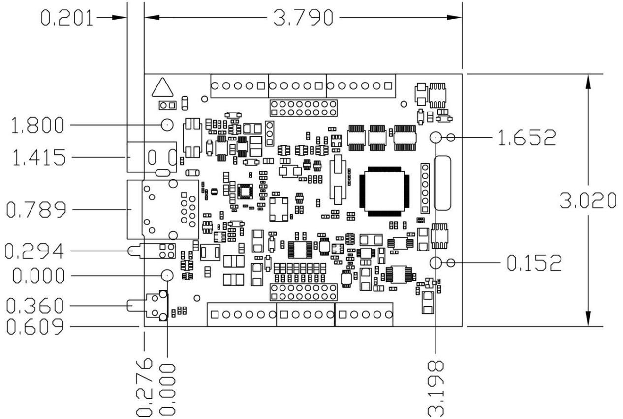
Figure 8. RedLab E-1608 device circuit board dimensions
