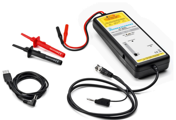
The R&S®RT-ZD01 high voltage differential probe provides 100 MHz bandwidth for up to 1400 V input voltage. Its BNC interface makes this probe ideal for the R&S®RTB2000.
