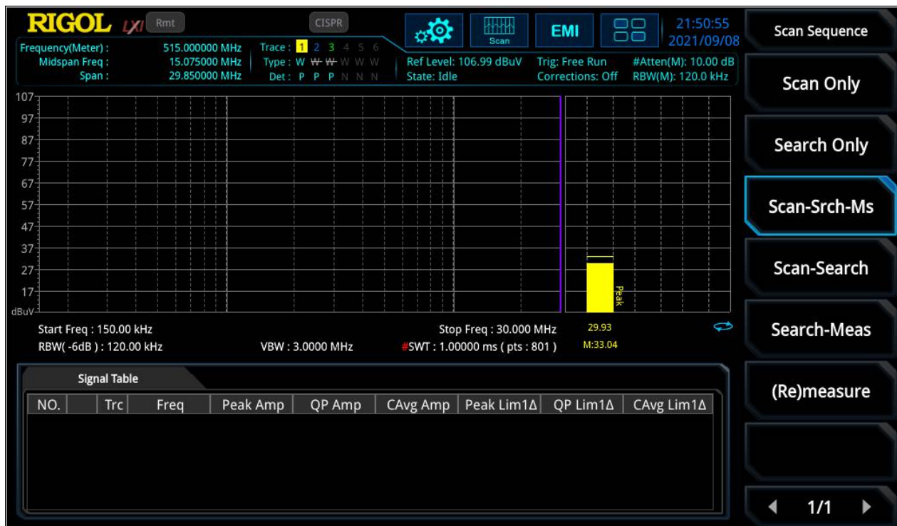
Figure 4: Scan Sequence adjustment with "Scan-Search-Measure"
