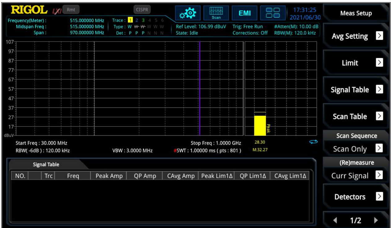
Figure 2: [Meas Setup] Window on right hand side
