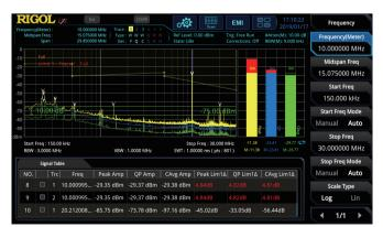
*Quickly recall the limit line compliant with the CISPR standard* (e.g. EN55011, EN55012, etc.) to carry out pre-test and monitor the target point with three different detectors.
