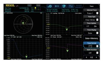
In VNA mode, you can make S11, S21, and DTF measurements for the components and circuit networks. The network characteristics of the components under test can be accurately demonstrated in Smith chart, Polar chart, and other formats.
